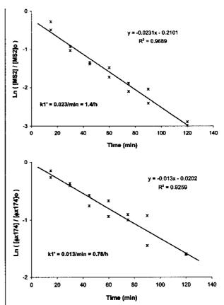
FIGURE 2. Pseudo-first-order removal of the bacteriophages MS-2 and  $\phi$ X174 in AGW in batch reactors containing 1.0 g of Peerless iron granules. Initial virus concentrations  $\approx 10^5$  pfu/mL. Shaking speed = 20 rpm.
