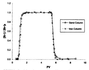
FIGURE 3. Breakthrough curves of bromide tracer from columns packed with oxide-removed sand only and oxide-removed sand plus iron granules.
