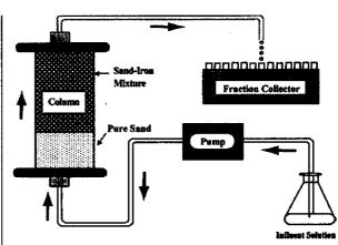
FIGURE 1. Schematic diagram of column experiment setup.
